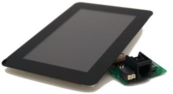
OnDutyDisplay is connected to OnDutyCore via the adapter supplied. The RJ12 cable required for this is not included in the scope of delivery. In addition, the power supply of the adapter must be established (see connection diagram on page 23).
